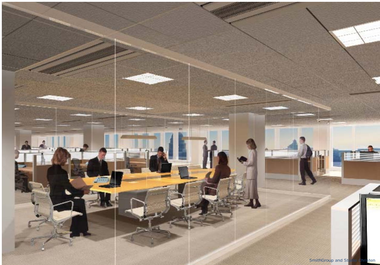
Figure 15: Rendering showing how the chilled beams will be incorporated into the ceiling grid.
